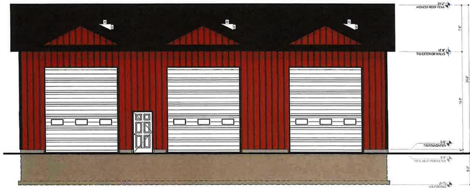
1 FRONT (EAST) ELEVATION SCALE: 1/4" = 1'-0"
